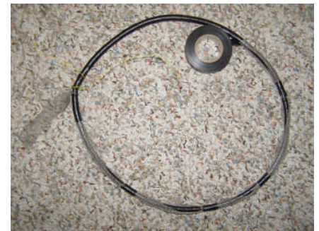
Fig. 7 Scotch 24 mesh shield being secured to coil with tape over second layer of spiral wrap.
