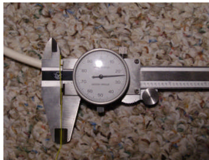
Fig. 1 Measuring OD of AWG 30 Teflon wire.
