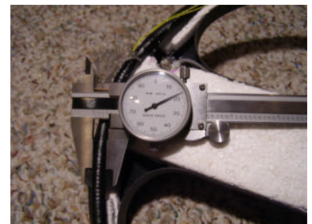
Fig. 2 Measuring the diameter of final shielded coil bundle.
