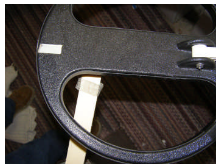
Fig. 6 Piece of Scotch 24 shield material held by a wood stick being tested.
